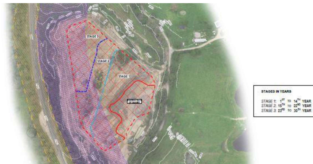
Figure: 2 – BSE plan of extraction stages showing estimated minimum distances of stage to Princes Highway road reserve.
